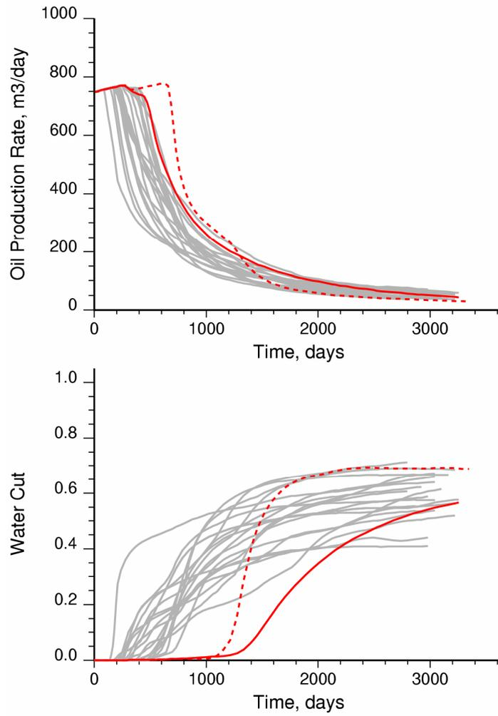
**Figure 16:** The solid red lines are the flow simulation results from a simplistic layercake model. The dashed lines are from an interpolated (kriged) model. The gray lines show the results from 20 geostatistical simulations.
