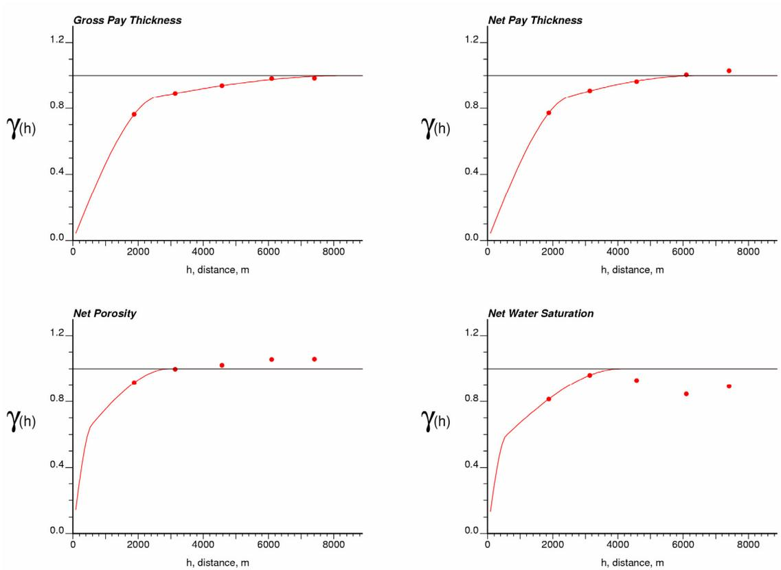
**Figure 8:** Variograms of the four variables under consideration. The dots are the calculated points and the solid line is the fitted curve. These variograms are isotropic.
