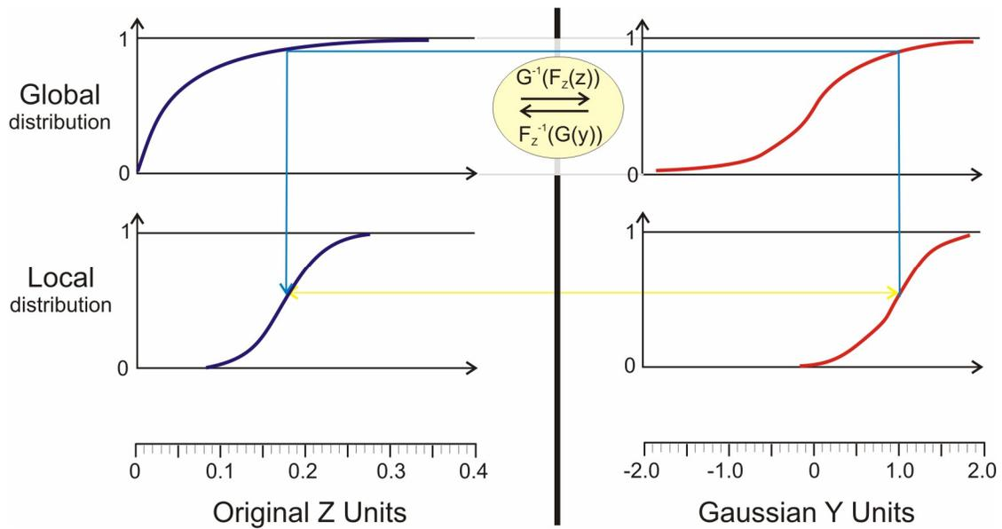
**Figure 2:** Schematic illustration of normal score transform. The original Z- data are on the left and the Gaussian Y-values are on the right. The top figures are the global CDFs and the bottom figures represent local CDFs. Quantiles are transformed using the global distribution (the three part blue line).
