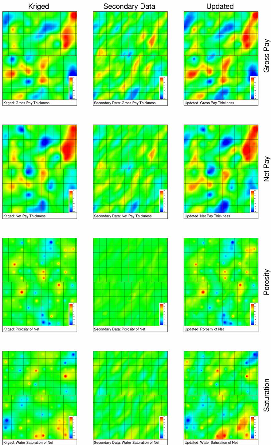
**Figure 9:** Each row shows maps of a variable being predicted. The map on the left is from well data alone, the center map is from secondary structural information, and the map on the right is updated map accounting for well and secondary data. The maps are in Gaussian units.
